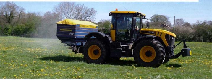
Self-levelling suspension front and rear ensures a smooth ride in the field and on the road with the big Bogballe spreader on the three-point linkage.
